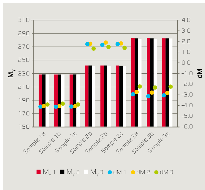
Figure 4: Jetness ( M_y ) and undertone (dM) of samples 1 to 3, measured using the 45°/0° tabletop instrument at three different spots a, b, c. For each spot, three mean values were determined from five measurements each: M_y and dM 1,2,3.
